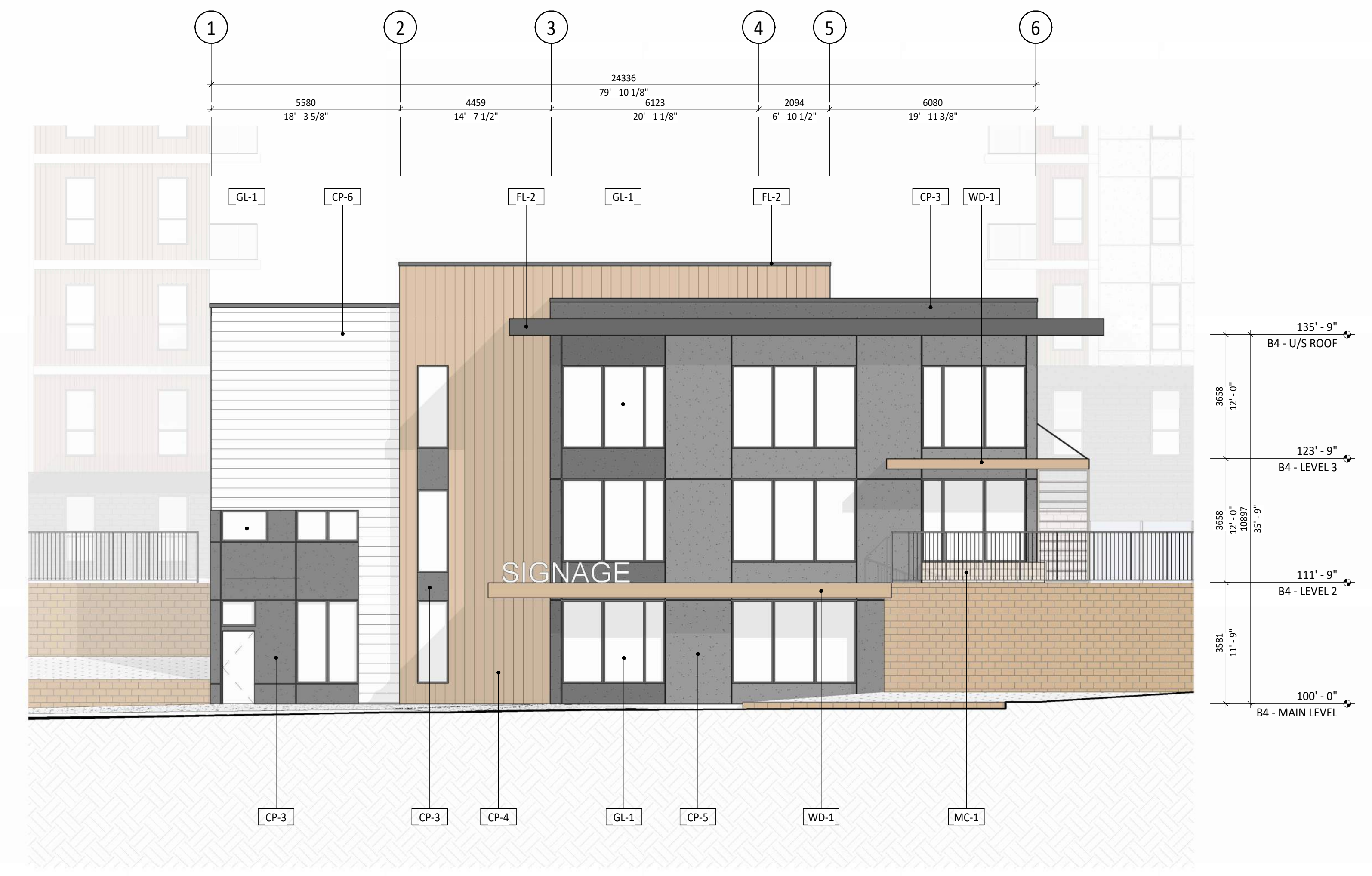
4 WEST ELEVATION DP40.01 1/8" = 1'-0"
