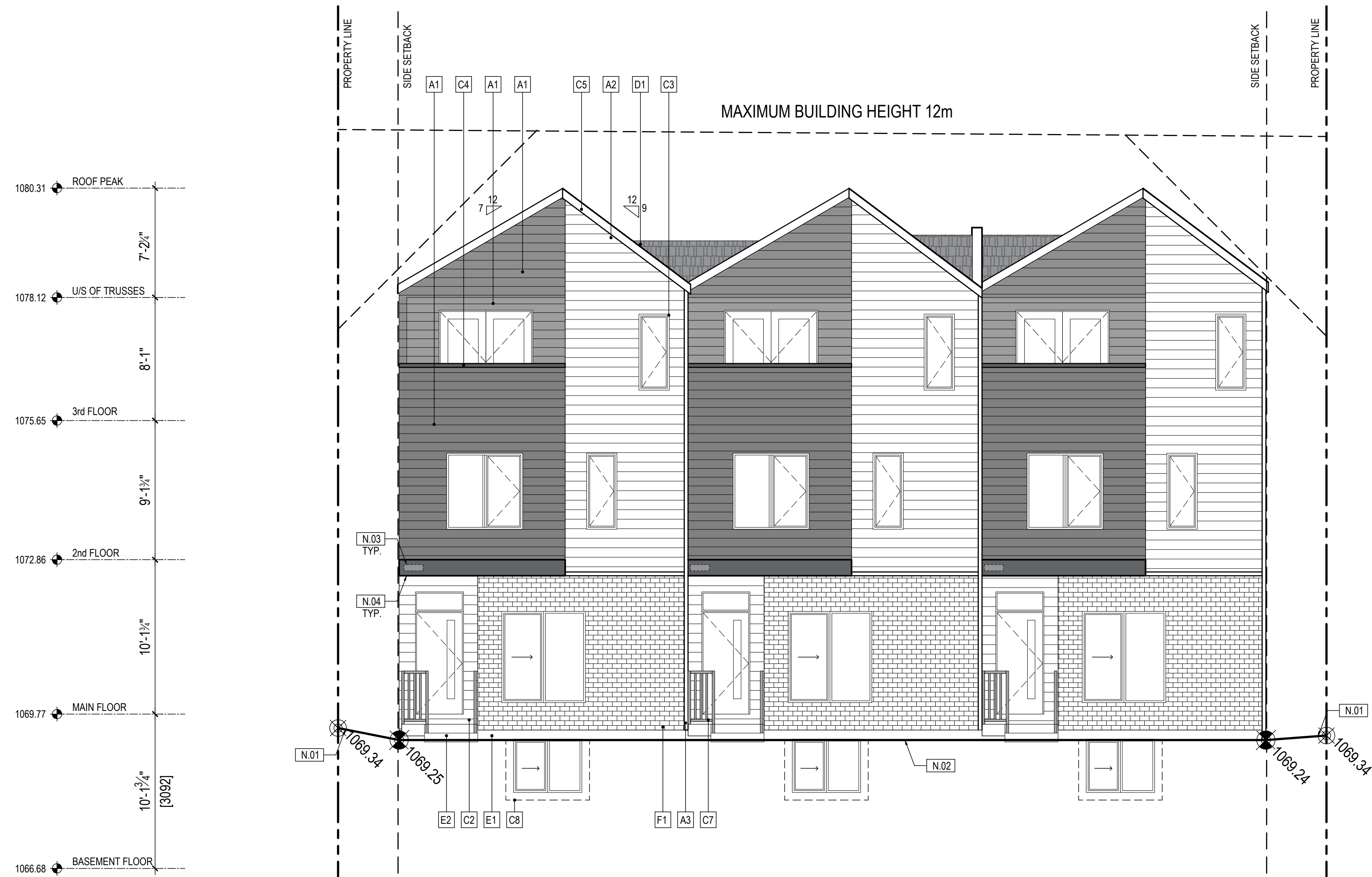
1 WEST ELEVATION - BLDG A DP.200 3/16" - 1'-0"
